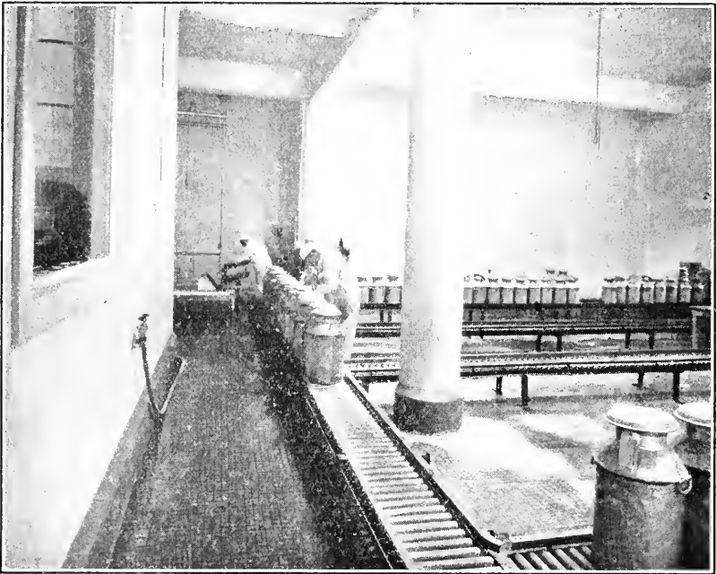
FIGURE 1.—Receiving milk at a plant using system 6. At 23 plants using systems similar to this an average of 2,334.4 gallons per hour and 459.6 gallons per man-hour was received
